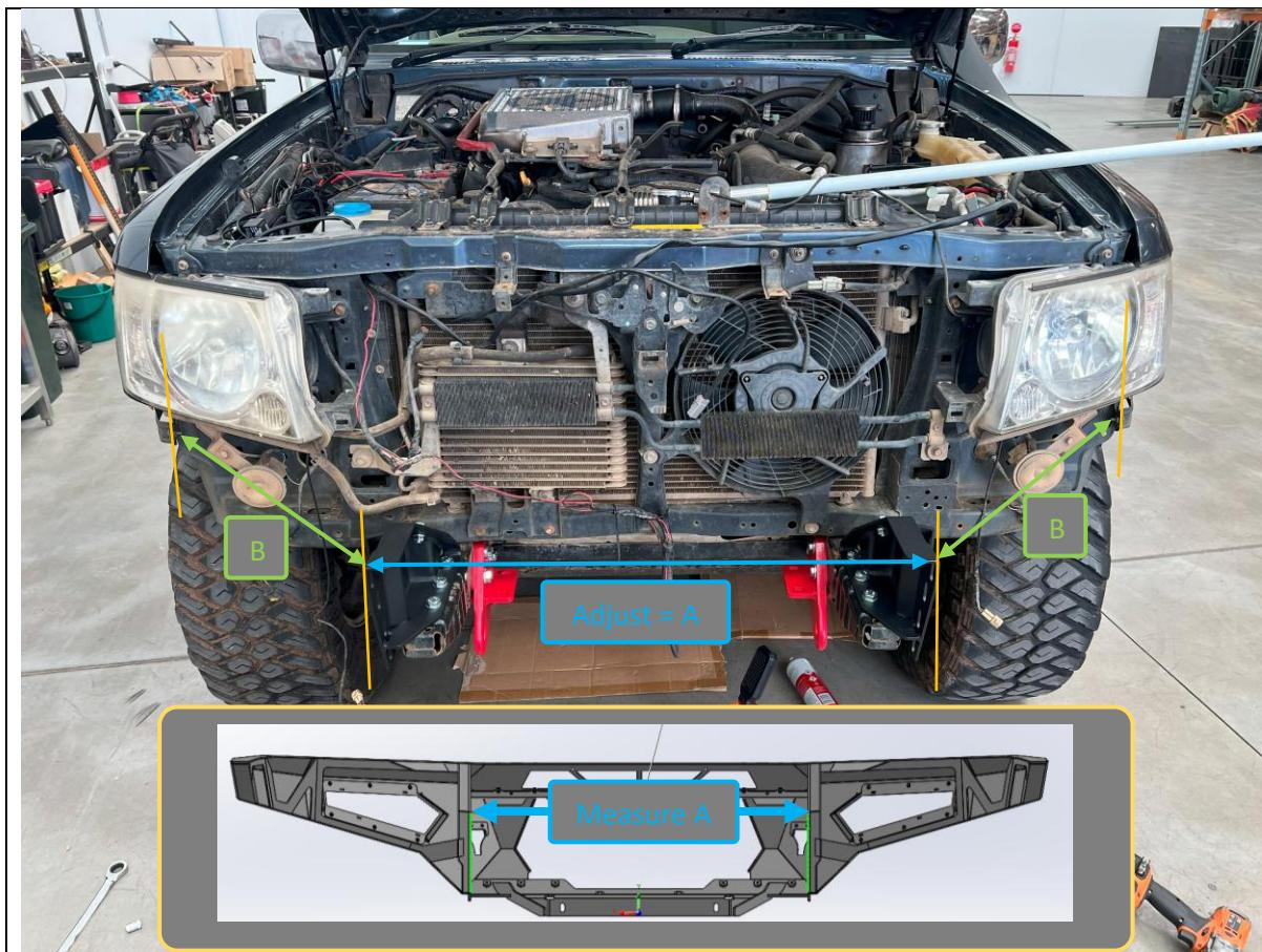
50. Time to adjust the Impact Assemblies. First measure the **INSIDE** distance between the uprights. This is Dimension A. You can write it below for Reference.
