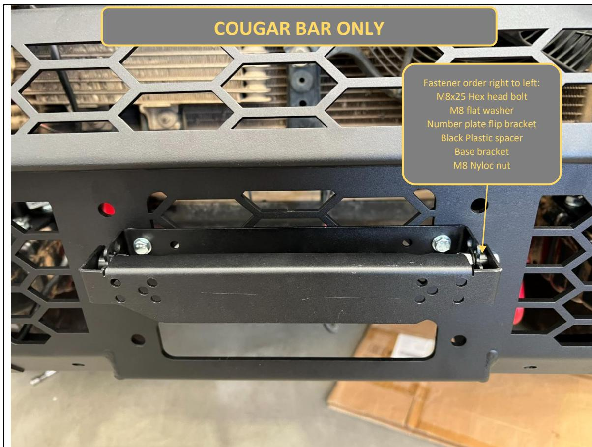
86. Assemble the Number plate flip. Ensure the fasteners are in the correct order as shown in the image above.
