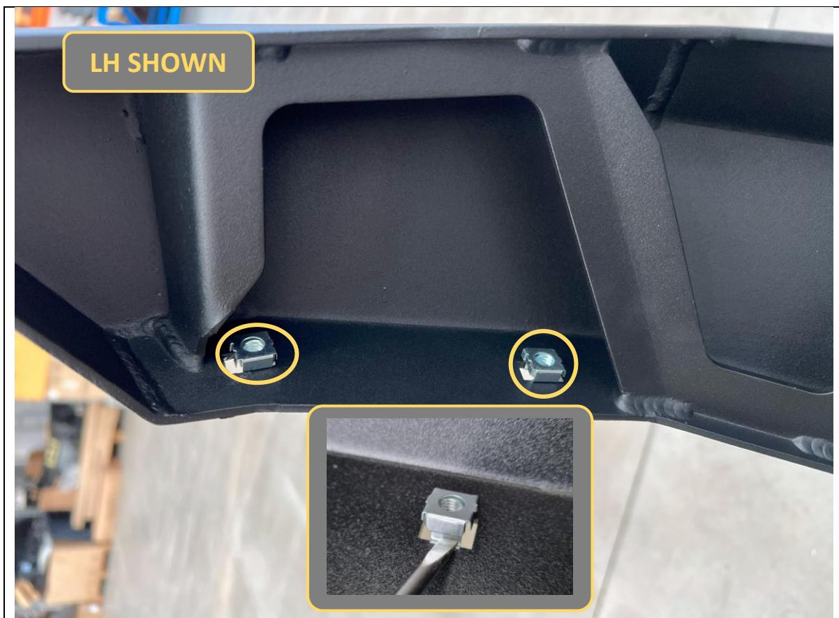
68. Fit 12x M6 cage nuts into the rectangular slots on the bottom of the bar wing (6x per side).
