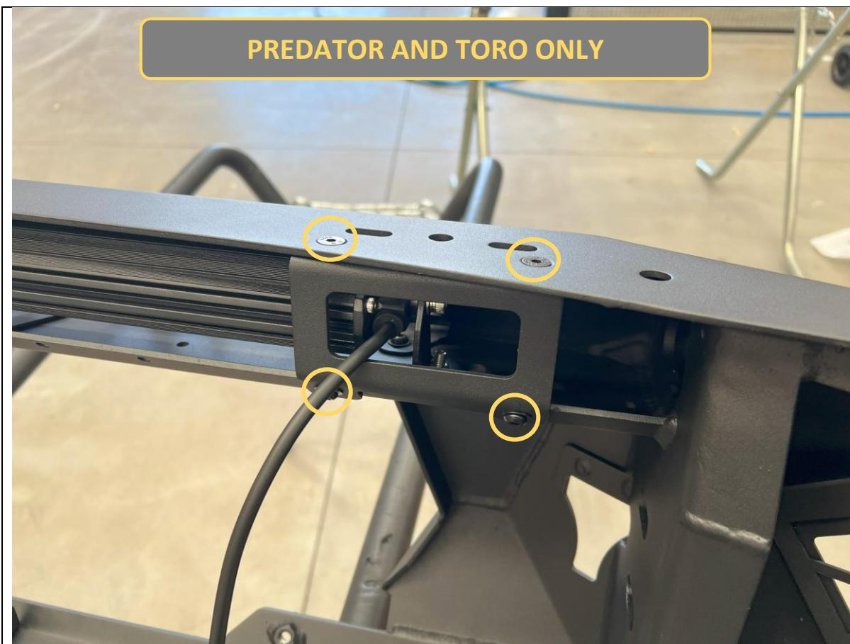
60. Fit the pan brace to the back of the middle section of the bar.
