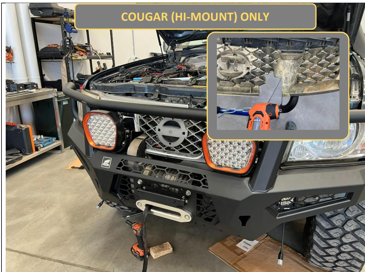
103. Using a power tool suitable for plastic cutting (we recommend a oscillating multi tool), Trim the area marked in the previous step.
