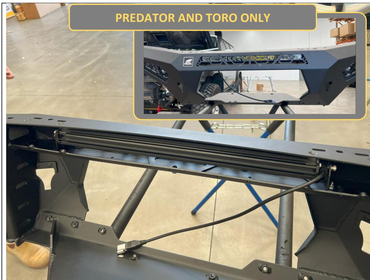
59. If fitting an integrated light bar, do so now from the back.
